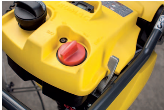
Integrated On/Off safety switch.
